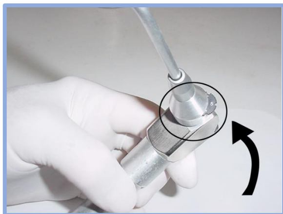
Figure 3. Photograph of a Fluid Control Block (FCB) with 5 choices of air volumes. Reprinted by permission of the copyright holder- IGI Global, Handbook of Research on Computerized Occlusal Analysis Technology Applications in Dental Medicine , pg. 443.
